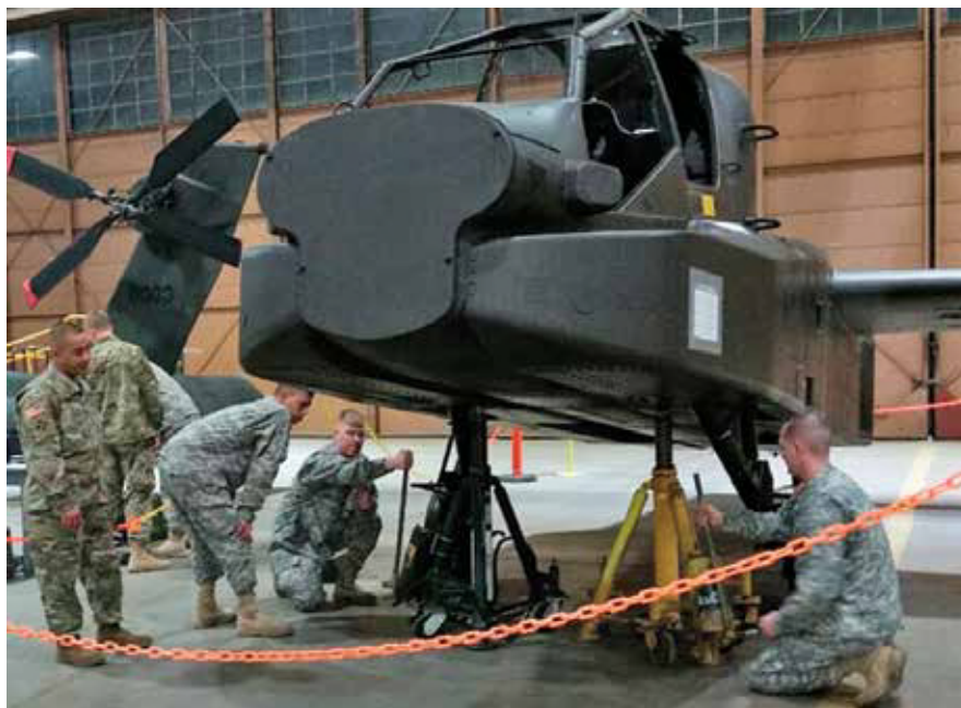
15R students from A/1-222d Avn. Regt. training with the new AH-64D landing gear trainer.
